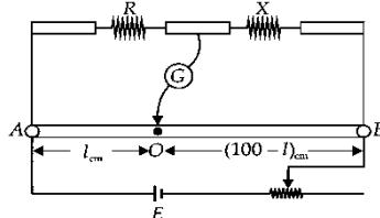
24. Potential gradient of potentiometer wire  $AB$  is  $K = \frac{V_{AB}}{L_{AB}}$
