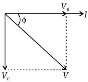
9.  $L - C - R$  circuit voltage and current
