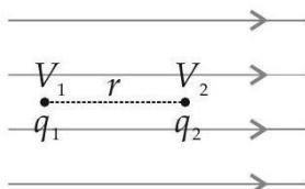
$$U = q_1 v_1 + q_2 v_2 + \frac{1}{4\pi\epsilon_0} \frac{q_1 q_2}{r}$$
